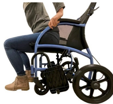
Figure 6 Incorrect posture – centre of gravity shifted too far forward and front wheels not aligned to the front.
