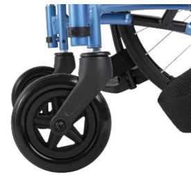
Figure 4 Correct caster position to the front
